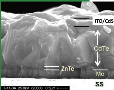
**SEM image of CdTe solar cell cross section showing layer composition.**
